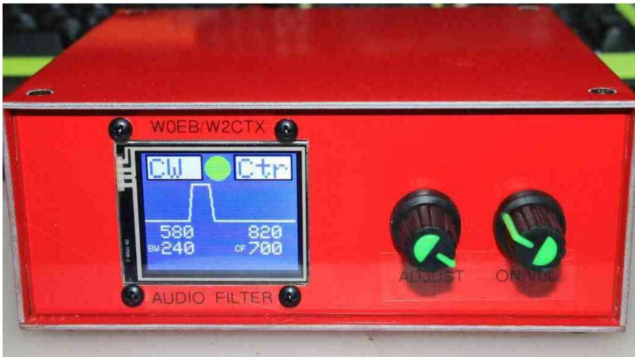
W0EB's build of the filter with the 1.8" Color touch Screen showing the adjustable CW filter. Green dot - CW Zero Beat indicator when incoming tone matches the filter's Center Frequency.
