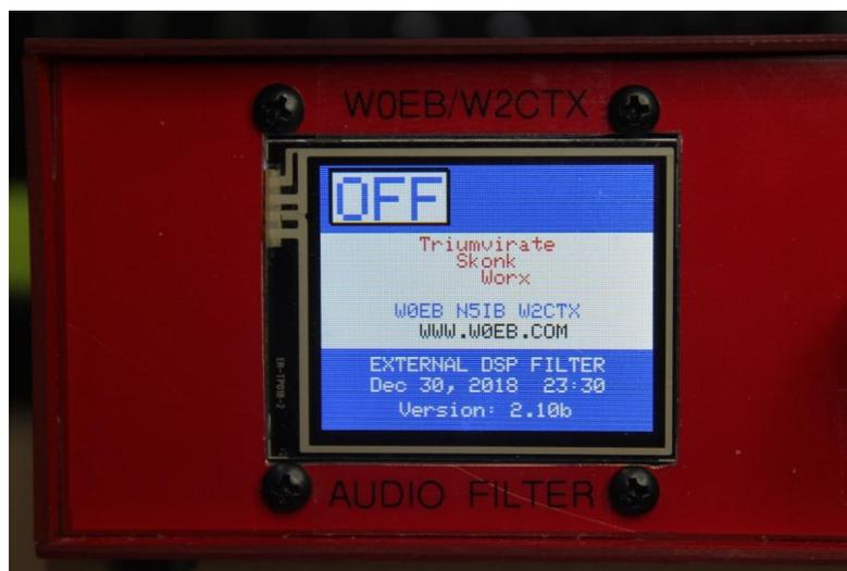
While this screen is displayed, the filter's effective bandwidth is 60-3000 Hz
