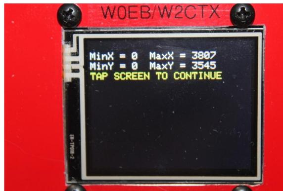
Tap the stylus on the screen and the Touch "X-Y" calibration will be complete. Now the "Splash Screen" display shown below will appear.
